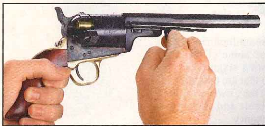
Conversions of the '51 Navy, such as this .38 Spl. by Traditions, generally employ an ejector rod on the right side of the revolver.
